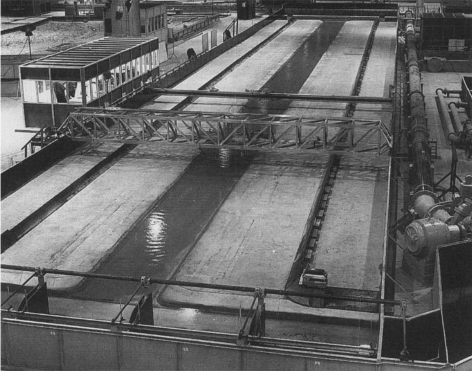
FIGURE 3. General view of a straight two-stage channel moulded in the Science and Engineering Research Council Flood Channel Facility (SERC-FCF) at Hydraulics Research Ltd, Wallingford. (Courtesy of Hydraulics Research Ltd.)
